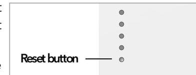
This button is below the LEDs on the front of the device.
